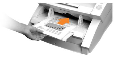
The document tray will stay up as long as the Bypass Mode key is lit. After scanning has been completed, press the Bypass Mode key to lower the document tray.
